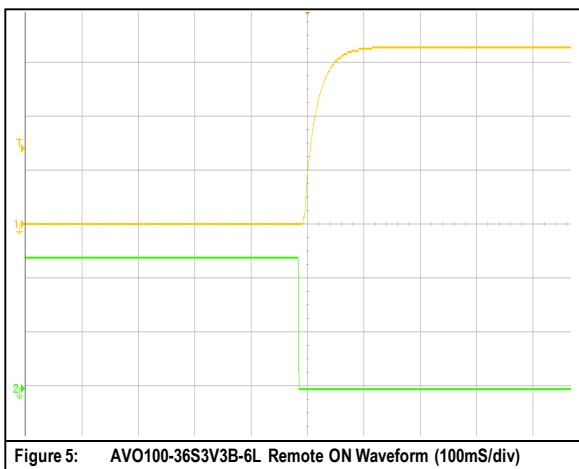
Figure 5: AVO100-36S3V3B-6L Remote ON Waveform (100mS/div)
