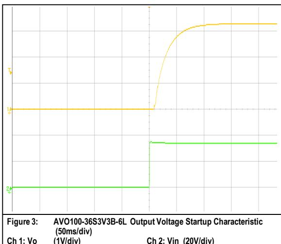
Figure 3: AVO100-36S3V3B-6L Output Voltage Startup Characteristic
