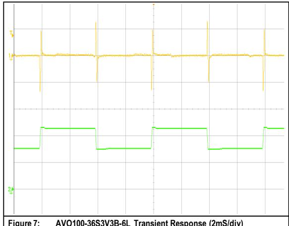
Figure 7: AVO100-36S3V3B-6L Transient Response (2mS/div)
