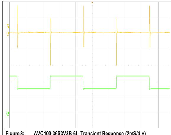
Figure 8: AVO100-36S3V3B-6L Transient Response (2mS/div)
