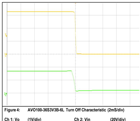
Figure 4: AVO100-36S3V3B-6L Turn Off Characteristic (2mS/div)
