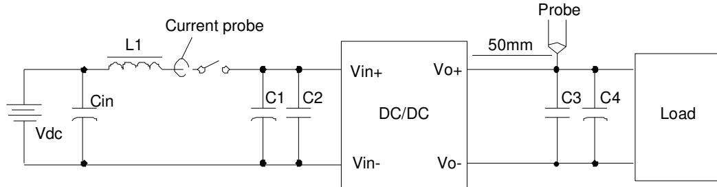
Figure 23 Input ripple &amp; output ripple &amp; noise test configuration
