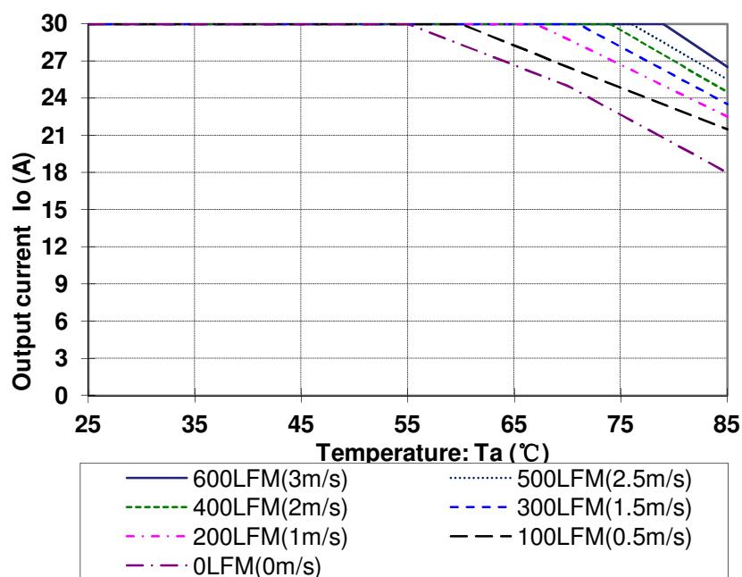
Figure 15 Output power derating, 24V<sub>in</sub>, air flowing across the converter from pin 3 to pin1
