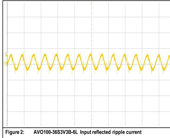
Figure 2: AVO100-36S3V3B-6L Input reflected ripple current
