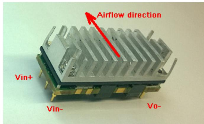
Figure 13 Typical test condition, heatsink size (L\*W\*H): 57.9mm\*22.86\*12.7mm
