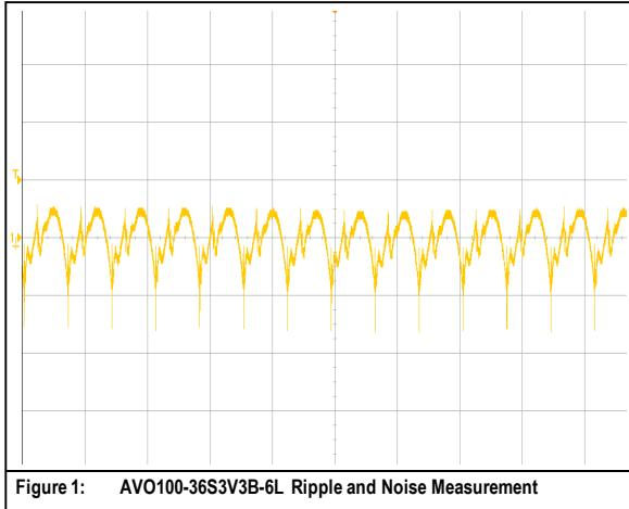
Figure 1: AVO100-36S3V3B-6L Ripple and Noise Measurement
