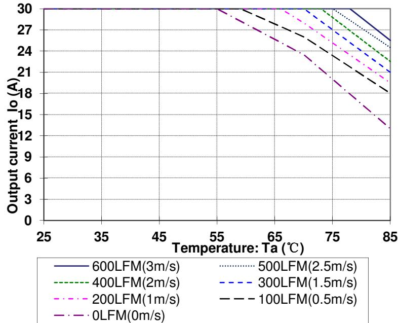
Figure 16 Output power derating,  $48V_{in}$ , air flowing across the converter from pin 3 to pin 1
