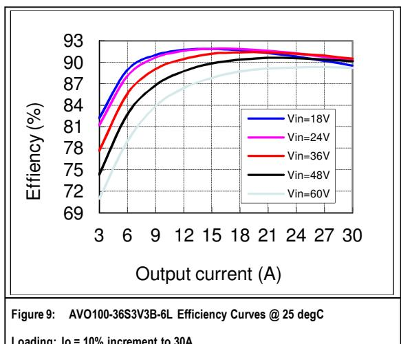
Figure 9: AVO100-36S3V3B-6L Efficiency Curves @ 25 degC
