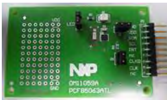
Fig 8. Picture of PCF85063ATL demo board OM11059A
