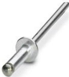
Blind rivets, Ø 2.4 mm, 8 mm sleeve length, aluminum sleeve, zinc-plated steel pin, special version with extended pin for fixing UW/RW/PW 4... (the UNIFOX-RVT M/BIT 2,4L nosepiece is required for processing)
