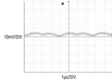
Figure 4. 2.5V LDO Output Ripple
