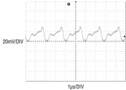
Figure 3. 3.3V Buck Output Ripple
