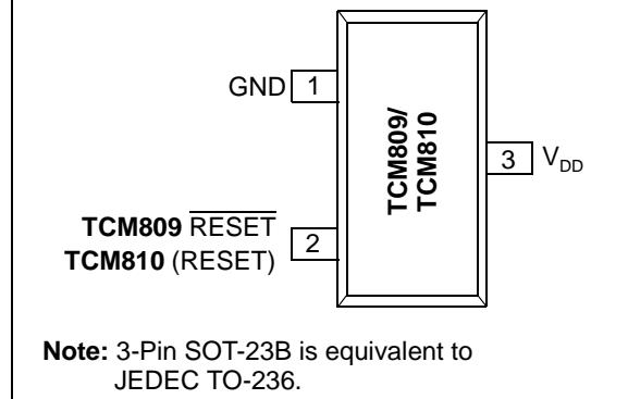
Note: 3-Pin SOT-23B is equivalent to JEDEC TO-236.
