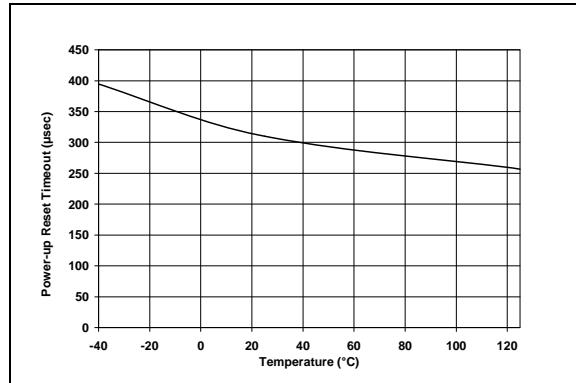
**FIGURE 2-3:** Power-up Reset Time Out vs. Temperature.
