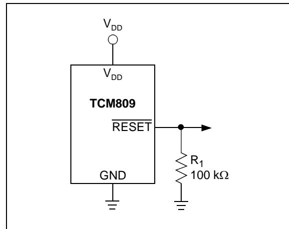
**FIGURE 4-2:** The addition of R<sub>1</sub> at the RESET output of the TCM809 ensures that the RESET output is valid to V<sub>DD</sub> = 0V.
