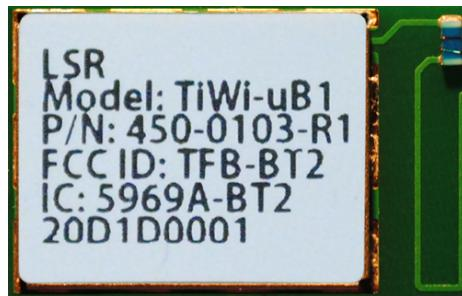
The TiWi-uB1 module fully supports the single mode *Bluetooth* Low Energy operation, and the output power can support class 3. The module provides the ability to either put your entire application into the integrated 8051 microcontroller, or use the module in Network Processor mode in conjunction with the microcontroller of your choice.
