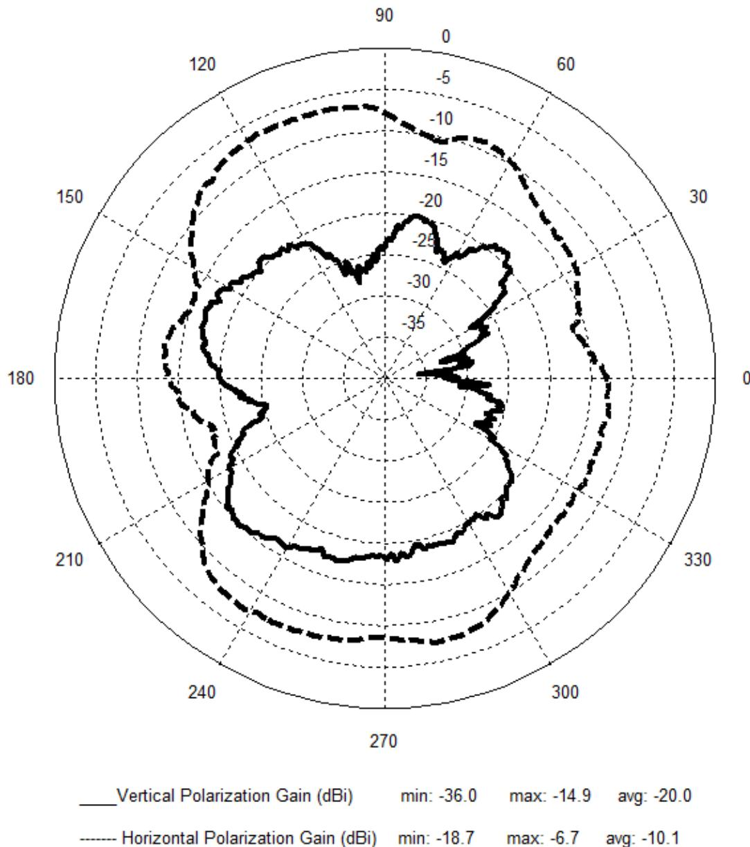
**Figure 14 PCB Trace Antenna Pattern (Flat @ 2440 MHz)**
