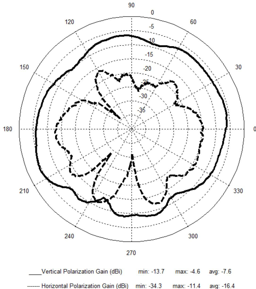
**Figure 13 PCB Trace Antenna Pattern (Horizontal @ 2440 MHz)**
