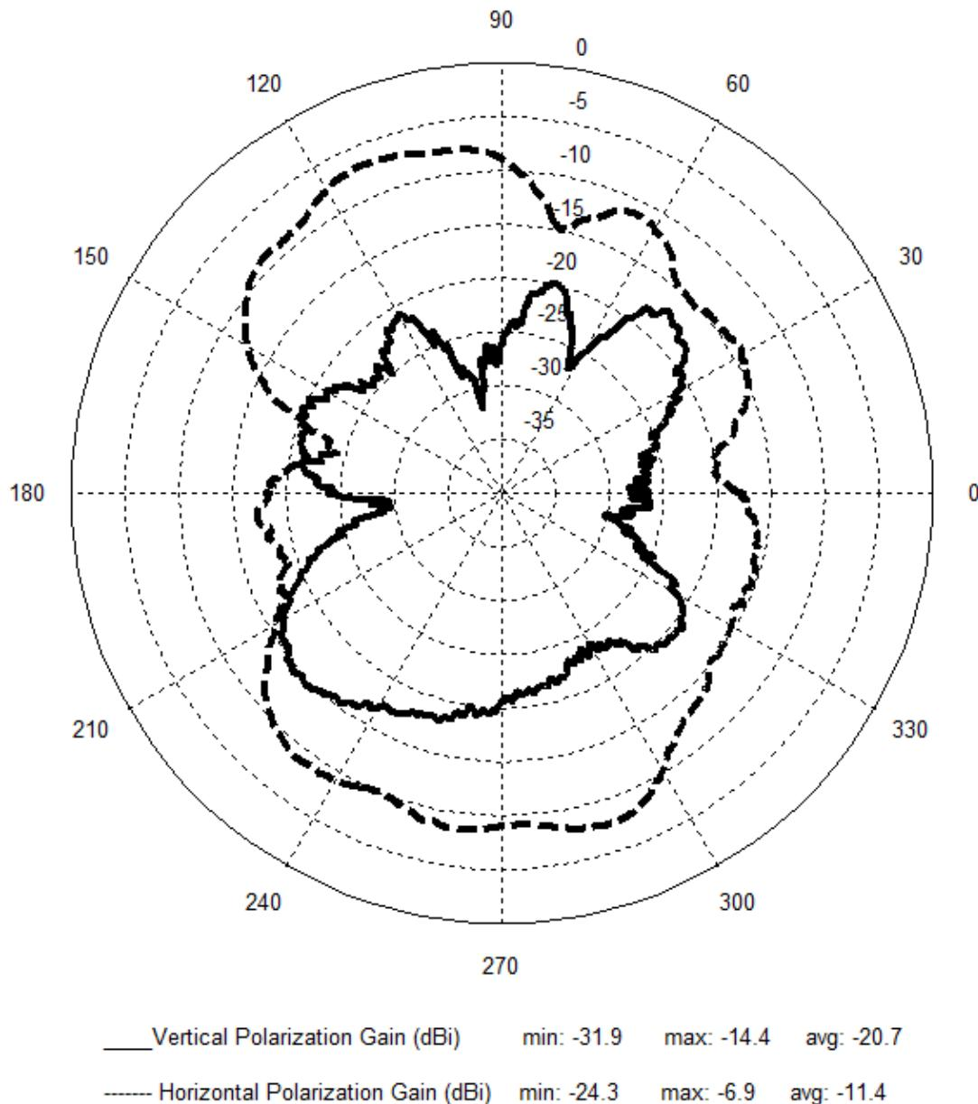
**Figure 11 PCB Trace Antenna Pattern (Flat @ 2405 MHz)**
