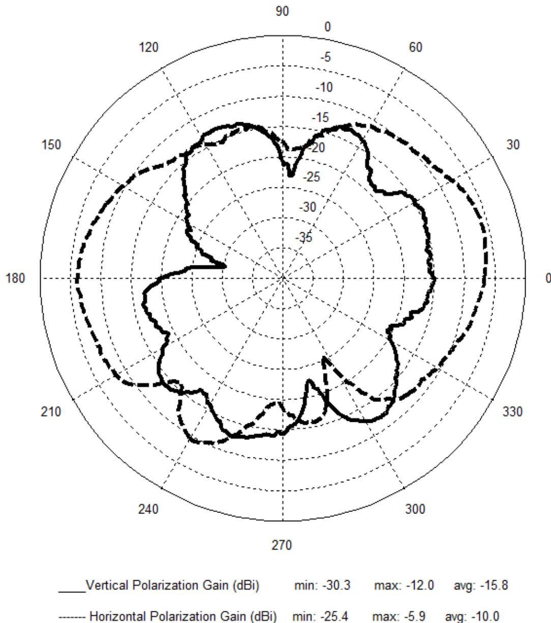
**Figure 12 PCB Trace Antenna Pattern (Vertical @ 2440 MHz)**
