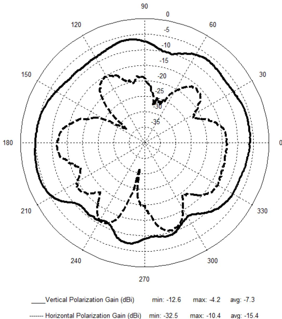
**Figure 16 PCB Trace Antenna Pattern (Horizontal @ 2480 MHz)**
