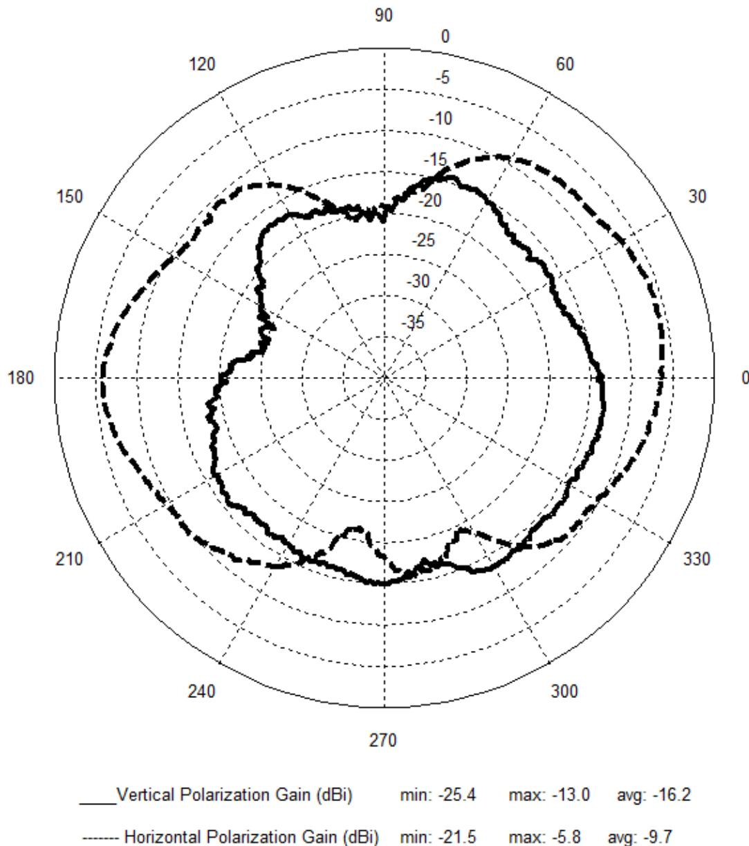
**Figure 15 PCB Trace Antenna Pattern (Vertical @ 2480 MHz)**
