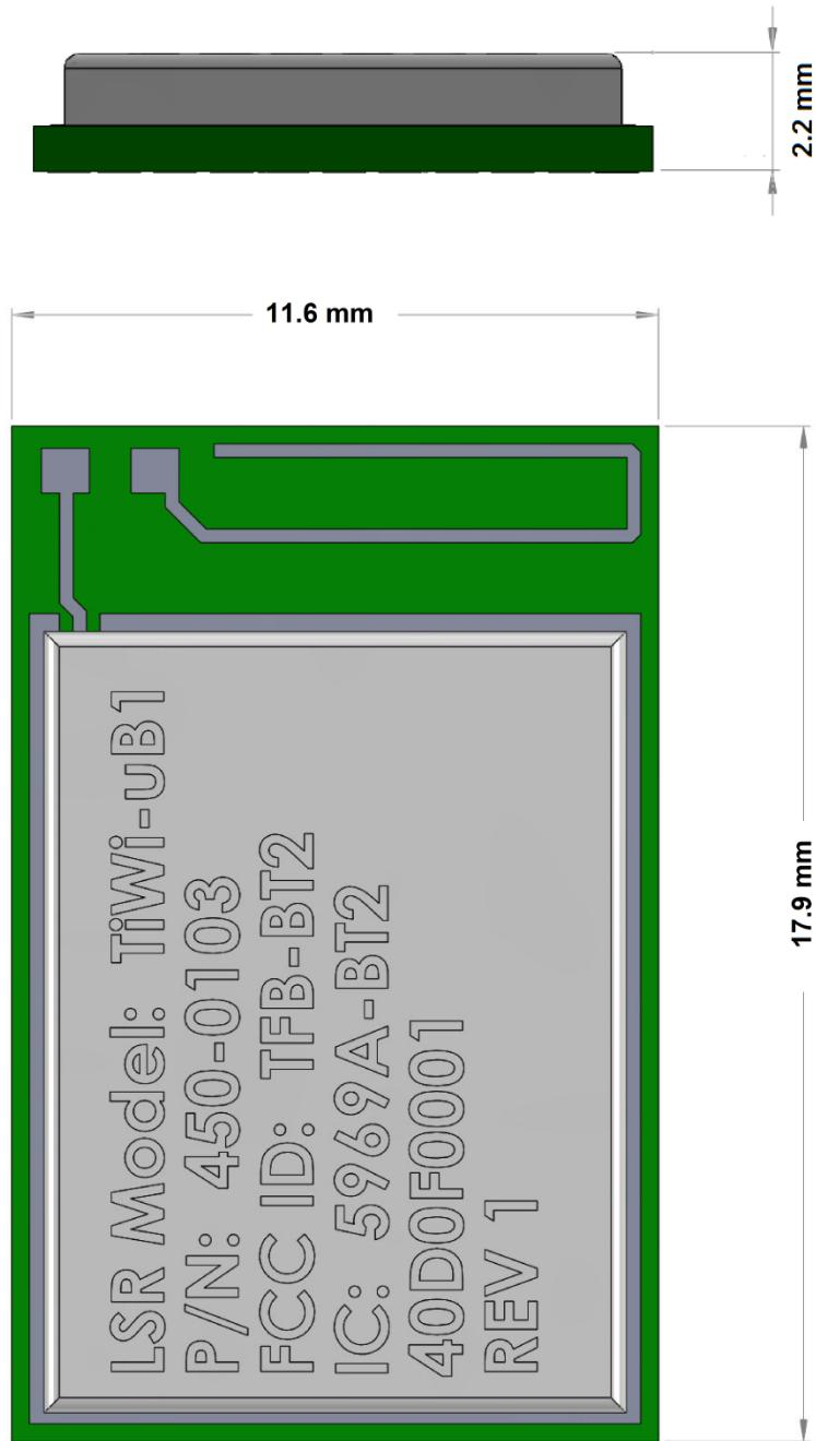
**Figure 18 Module Mechanical Dimensions (Maximum Module Height = 2.3mm)**
