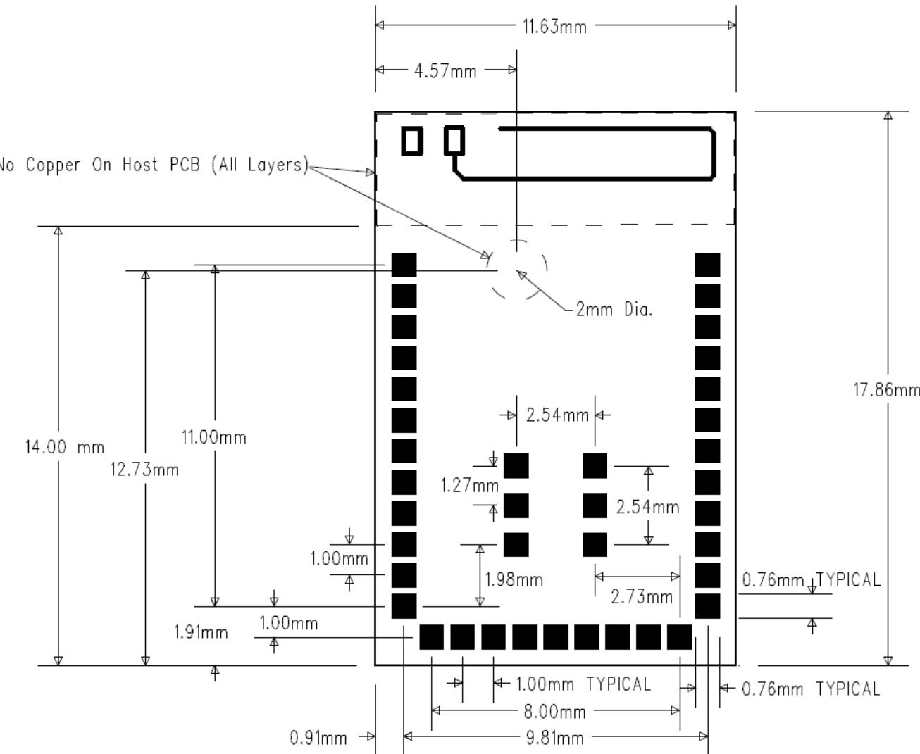
**Figure 19 TiWi-uB1 Recommended PCB Footprint (Viewed from Top)**
