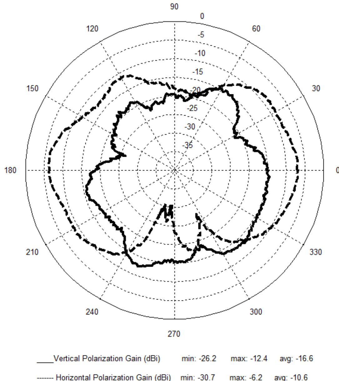
**Figure 9 PCB Trace Antenna Pattern (Vertical @ 2405 MHz)**
