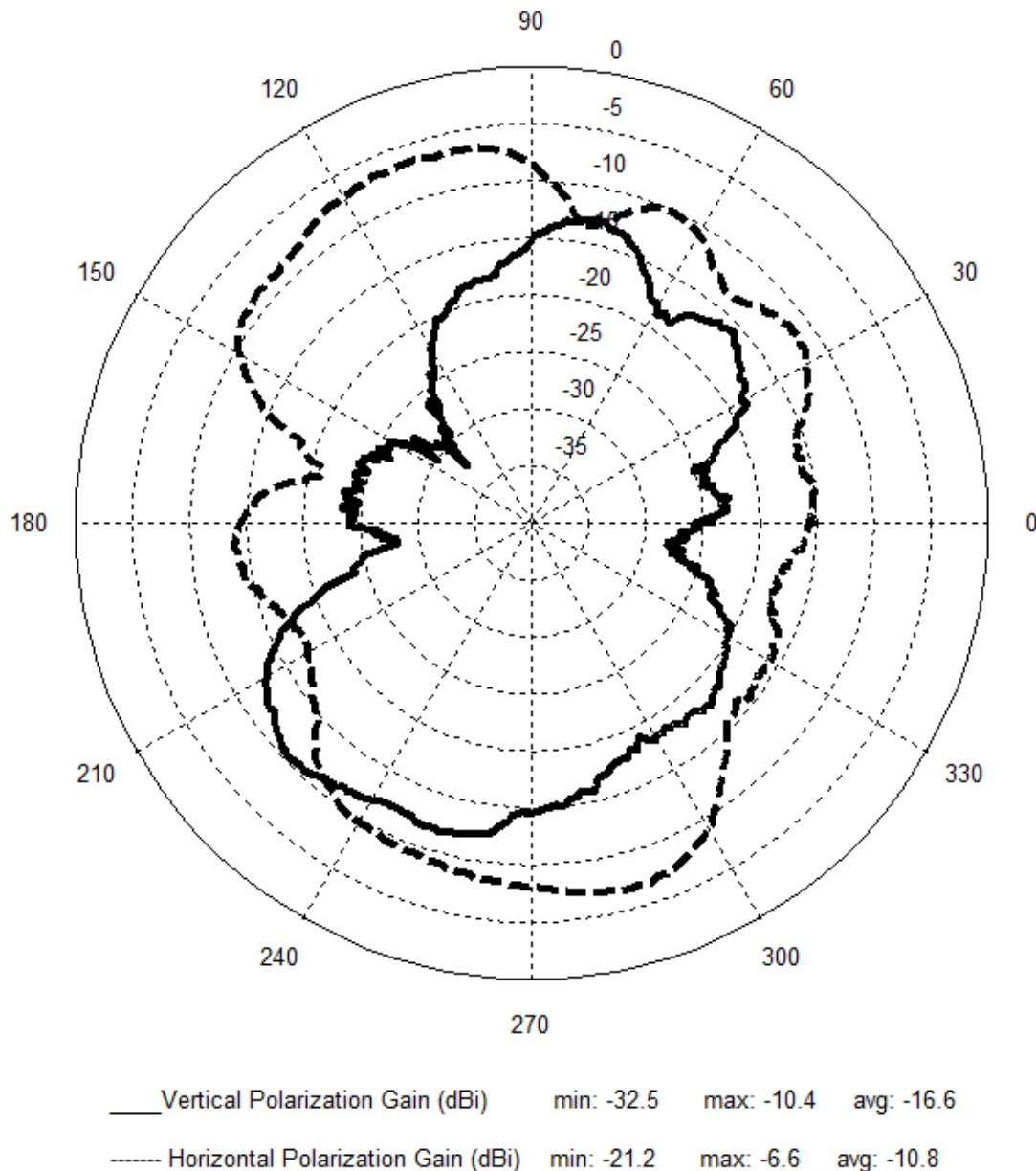
**Figure 17 PCB Trace Antenna Pattern (Flat @ 2480 MHz)**
