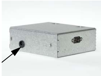
Figure 3-7 Low-voltage connector of the power supply unit
