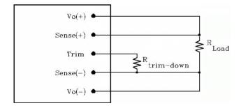
Figure 19: Circuit configuration for trim-down (decrease output voltage)
