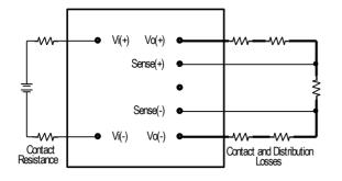
Figure 18: Effective circuit configuration for remote sense operation
