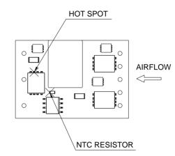
Figure 22: \* Hot spot& NTC resistor temperature measurement location. The allowed maximum hot spot temperature is defined at 120 %
