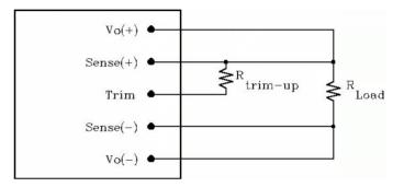
*Figure 20:* Circuit configuration for trim-up (increase output voltage)
