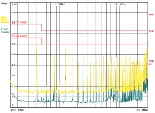
Figure 16 - EMI test positive line
