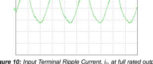
**Figure 10:** Input Terminal Ripple Current,  $i_{cr}$  at full rated output current and nominal input voltage with 12µH source impedance and 33µF electrolytic capacitor (200 mA/div, 1us/div)
