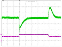
**Figure 8:** Output voltage response to step-change in load current (75%-50%-75% of lo, max; di/dt =  $0.1A/\mu$ s). Load cap: 10µF tantalum capacitor and 1µF ceramic capacitor. Top Trace: Vout (0.15V/div, 200us/div), Bottom Trace: lout (5A/div). Scope measurement should be made using a BNC cable (length shorter than 20 inches). Position the load between 51 mm to 76 mm (2 inches to 3 inches) from the module
