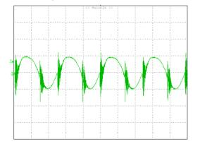
**Figure 13:** Output voltage ripple at nominal input voltage and rated load current (Io=7.5A)(50 mV/div, 1us/div) Load capacitance:  $1\mu$ F ceramic capacitor and  $10\mu$ F tantalum capacitor. Bandwidth: 20 MHz. Scope measurements should be made using a BNC cable (length shorter than 20 inches). Position the load between 51 mm to 76 mm (2 inches to 3 inches) from the module.
