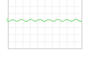
**Figure 11:** Input reflected ripple current,  $i_s$ , through a  $12\mu$ H source inductor at nominal input voltage and rated load current (20 mA/div, 2us/div)
