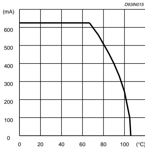
**Figure 7:** Max. Output Current vs. Ambient Temperature (SO20 Package,  $R_{th\ j\text{-amb}} = 90^\circ\text{C/W}$ )
