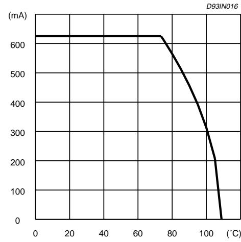
**Figure 8:** Max. Output Current vs. Ambient Temperature (SIP9 Package,  $R_{th\ j\text{-amb}} = 70^\circ\text{C/W}$ )
