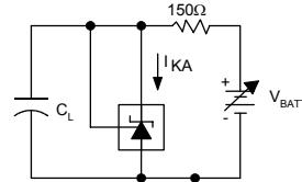
Test Circuit for Curve A
