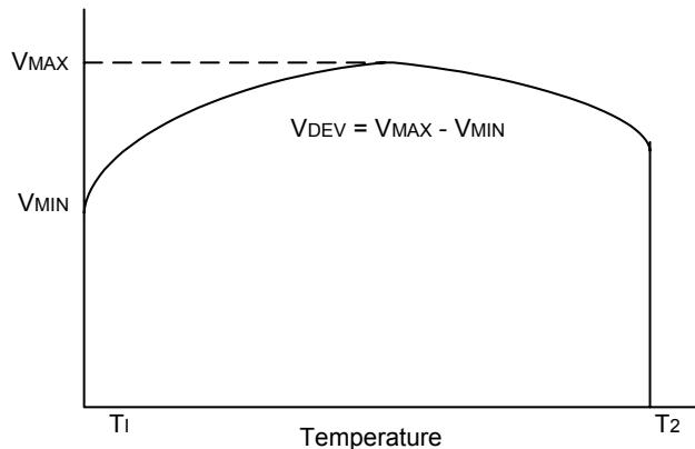
Note: 8. Deviation of reference input voltage,  $V_{DEV}$ , is defined as the maximum variation of the reference over the full temperature range. The average temperature coefficient of the reference input voltage  $\alpha V_{REF}$  is defined as:
