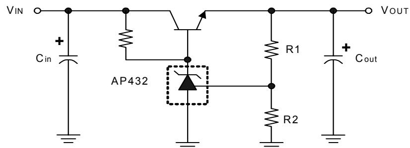
$$V_{OUT} = (1 + R_1/R_2)V_{REF}$$
