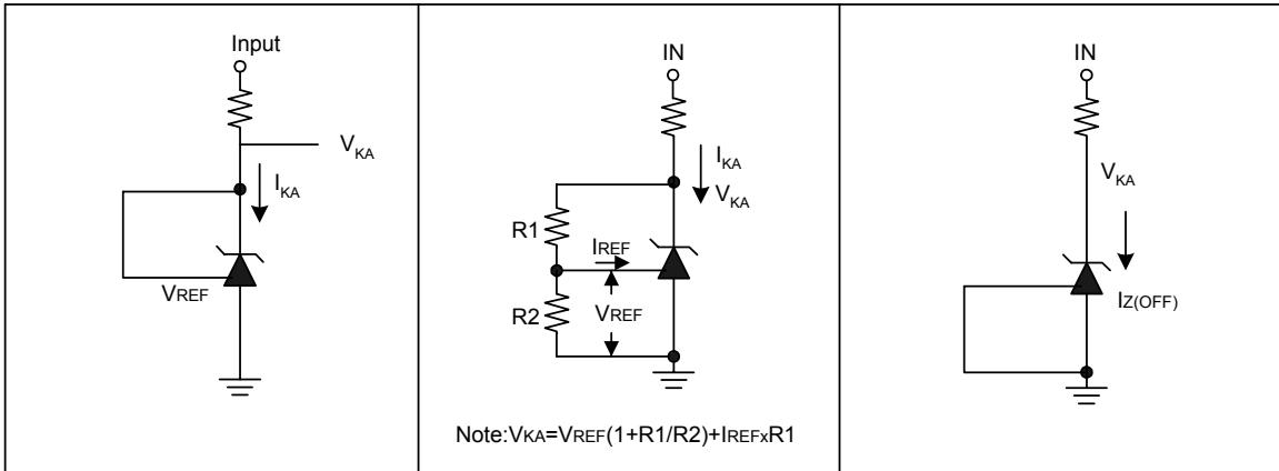
Fig 1. Test Circuit for  $V_{KA} = V_{REF}$
