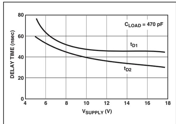
**FIGURE 2-6:** Propagation Delay Time vs. Supply Voltage.
