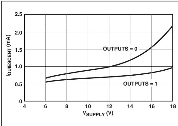
**FIGURE 2-8:** Quiescent Supply Current vs. Supply Voltage.
