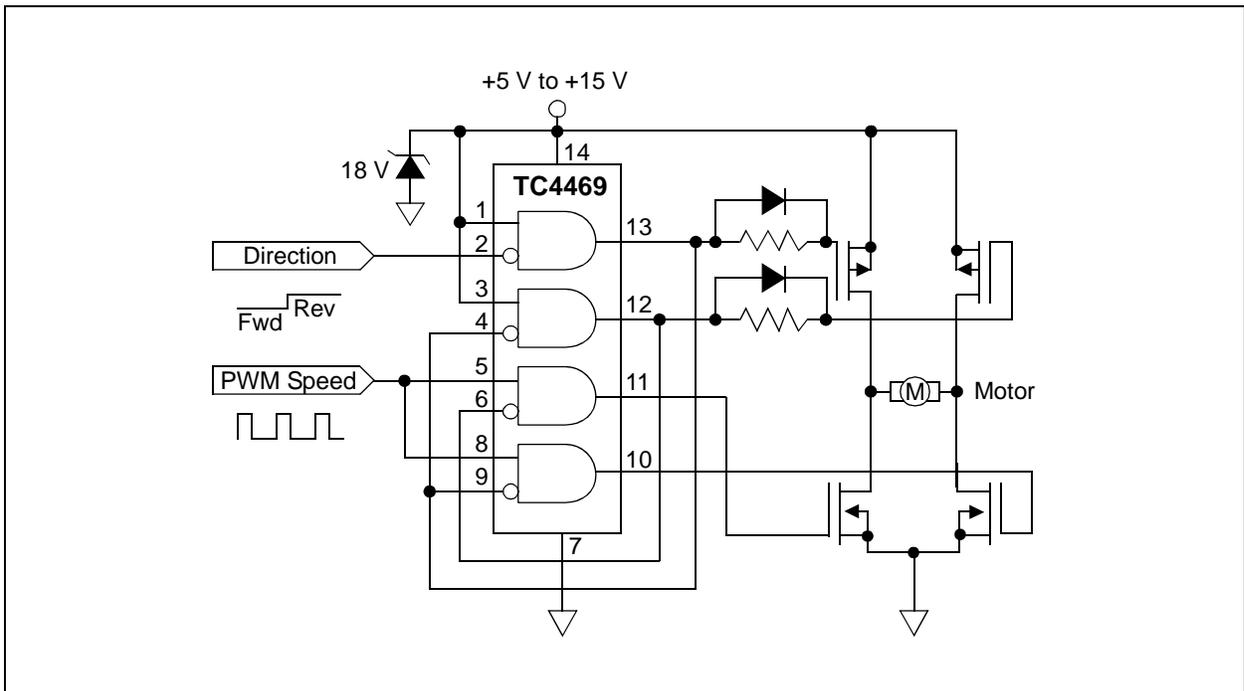
**FIGURE 5-2:** Quad Driver For H-bridge Motor Control.
