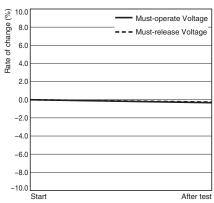
Characteristics were measured after applying a shock of 490 m/s² to the test piece 3 times each in 6 directions along 3 axes.
