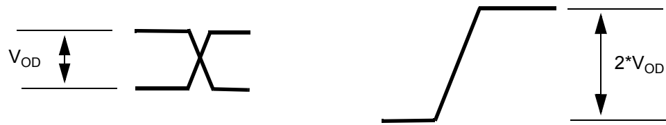
Figure 20 - Differential Voltage Parameter
