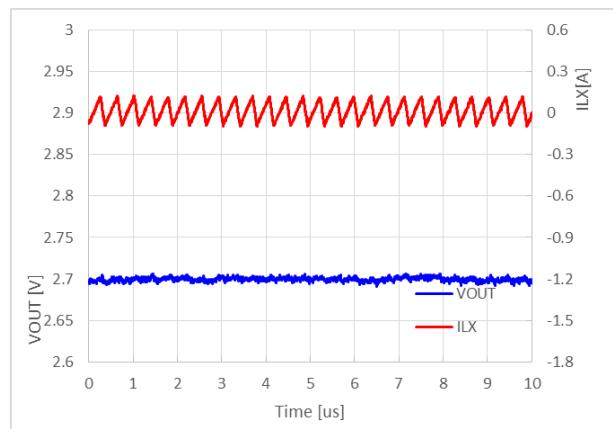
**RP602Z330x,  $V_{IN} = 3.6 \text{ V}$ , MODE = H
