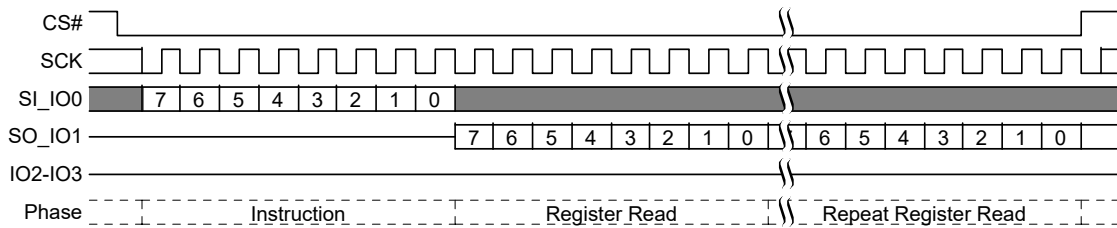
Figure 56. Read Configuration Register (RDCR) Command Sequence
