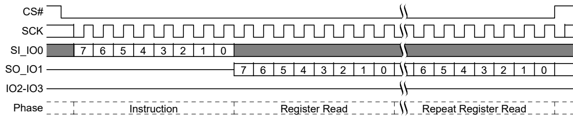
Figure 56. Read Configuration Register (RDCR) Command Sequence
