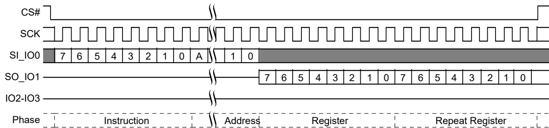
Figure 110. PPB Read Command Sequence
