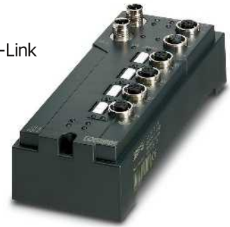
4 IO-Link ports and 4 digital inputs
