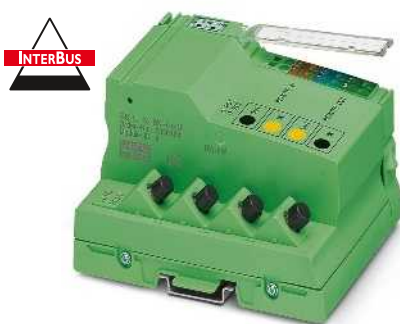
45° angled fiber optic connection
