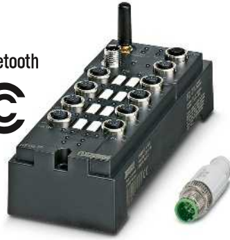
I/O wireless module, incl. OMNI antenna
