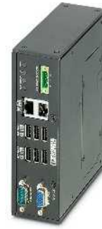
Box PC with extended temperature range
