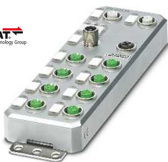
8 digital inputs and 4 digital outputs
