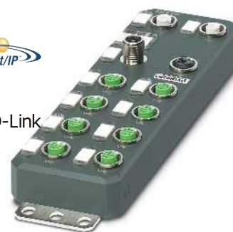
8 IO-Link ports, 4 digital inputs
