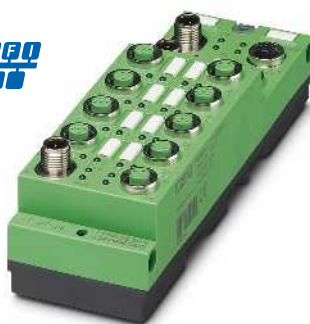
8 digital inputs and 8 digital outputs
