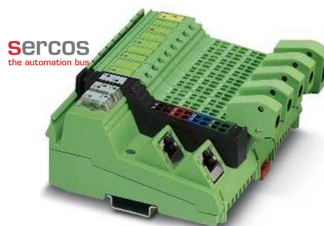
4 analog inputs and 2 analog outputs
