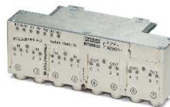
8 digital inputs and 8 digital outputs that can be read
