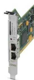
Router with firewall for PCI
