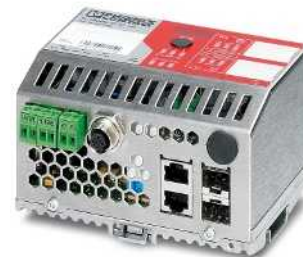
Gigabit router with firewall, replaceable memory
