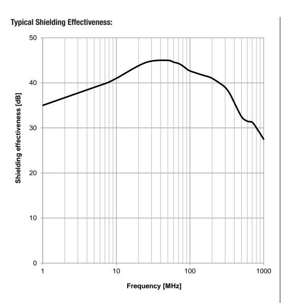
GENERAL TOLERANCE CREATED CHECKED Würth Elektronik eiSos GmbH & Co. KG EMC & Inductive Solutions KaS JoV DIN ISO 2768-1m Max-Eyth-Str. 1 74638 Waldenburg **WE-ST Conductive Ni/Cu glass** Tel. +49 (0) 79 42 945 - 0 fiber woven ORDER CODE www.we-online.com 30506 eiSos@we-online.com REVISION STATUS DATE (YYYY-MM-DD) BUSINESS UNIT PAGE 003.000 Valid 2016-12-30 eiSos 2/3 **WÜRTH ELEKTRONİK**
