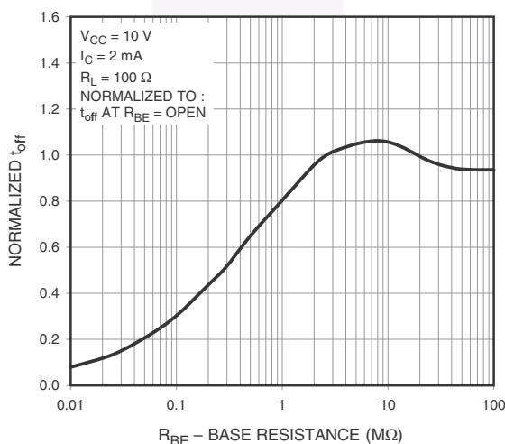
Figure 11. Normalized t<sub>off</sub> vs. R<sub>BE</sub>
