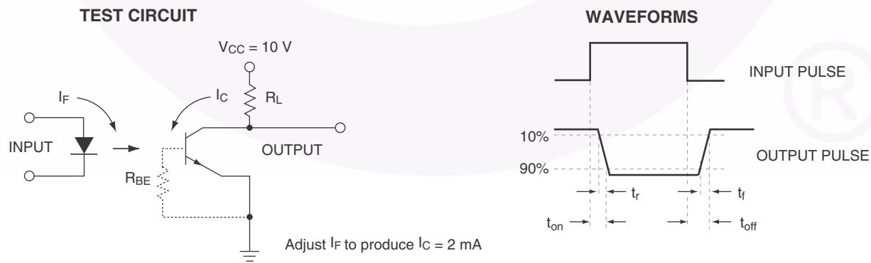
Figure 12. Switching Time Test Circuit and Waveforms
