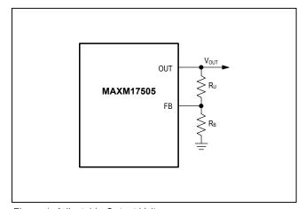
Figure 1. Adjustable Output Voltage
