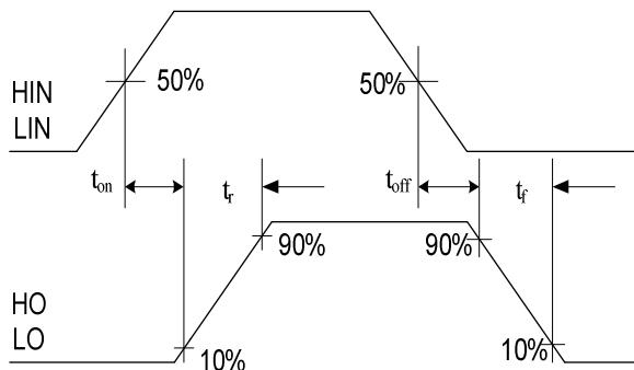
Figure 2. IC switching waveforms definitions.
