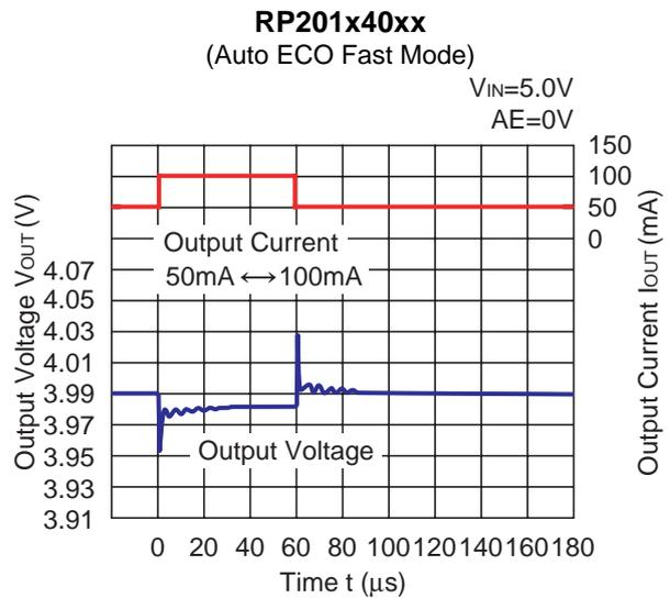
13) AE Switch Transient Response ( $C1=1.0\mu\text{F}$ ,  $C2=1.0\mu\text{F}$ ,  $t_r=t_f=0.5\mu\text{s}$ ,  $T_{\text{opt}}=25^\circ\text{C}$ )
