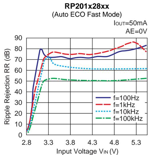
10) Ripple Rejection vs. Frequency (C1=none, C2=1.0μF, Ripple=0.2V<sub>p-p</sub>, T<sub>opt</sub>=25°C)
