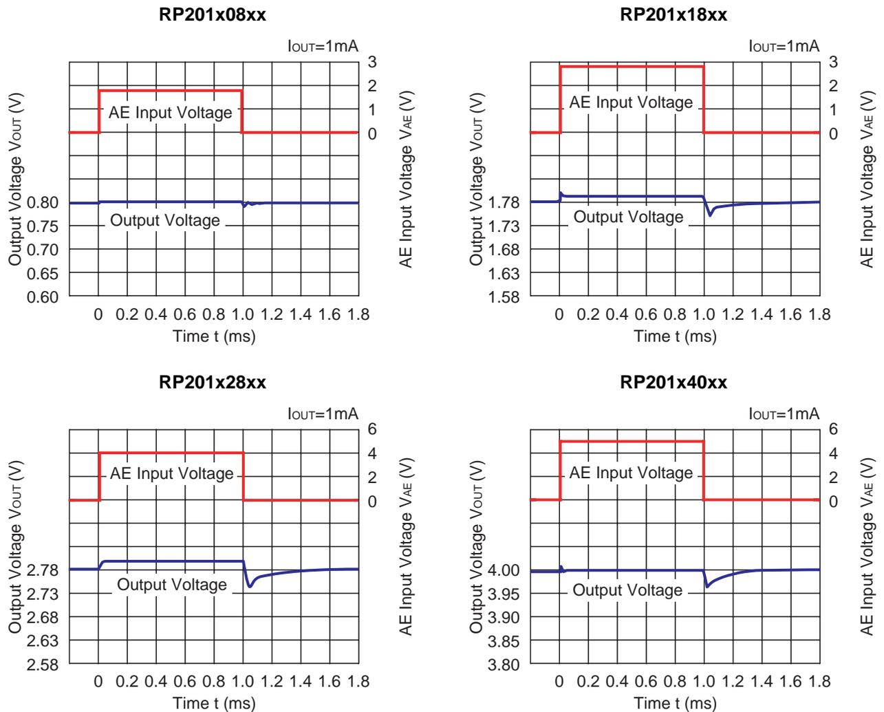
14) Turn On Speed with CE pin ( $C1=1.0\mu\text{F}$ ,  $C2=1.0\mu\text{F}$ ,  $T_{\text{opt}}=25^\circ\text{C}$ )
