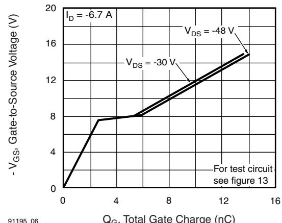
**Fig. 6 - Typical Gate Charge vs. Gate-to-Source Voltage**
