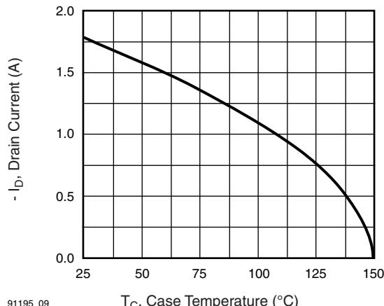
**Fig. 9 - Maximum Drain Current vs. Case Temperature**
