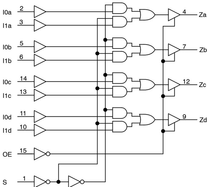
**Figure 2. Logic Diagram**
