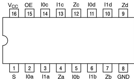
**Figure 1. Pinout: 16-Lead Plastic Package (Top View)**
