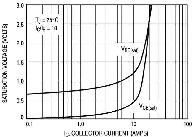
Figure 5. Typical Saturation Voltages
