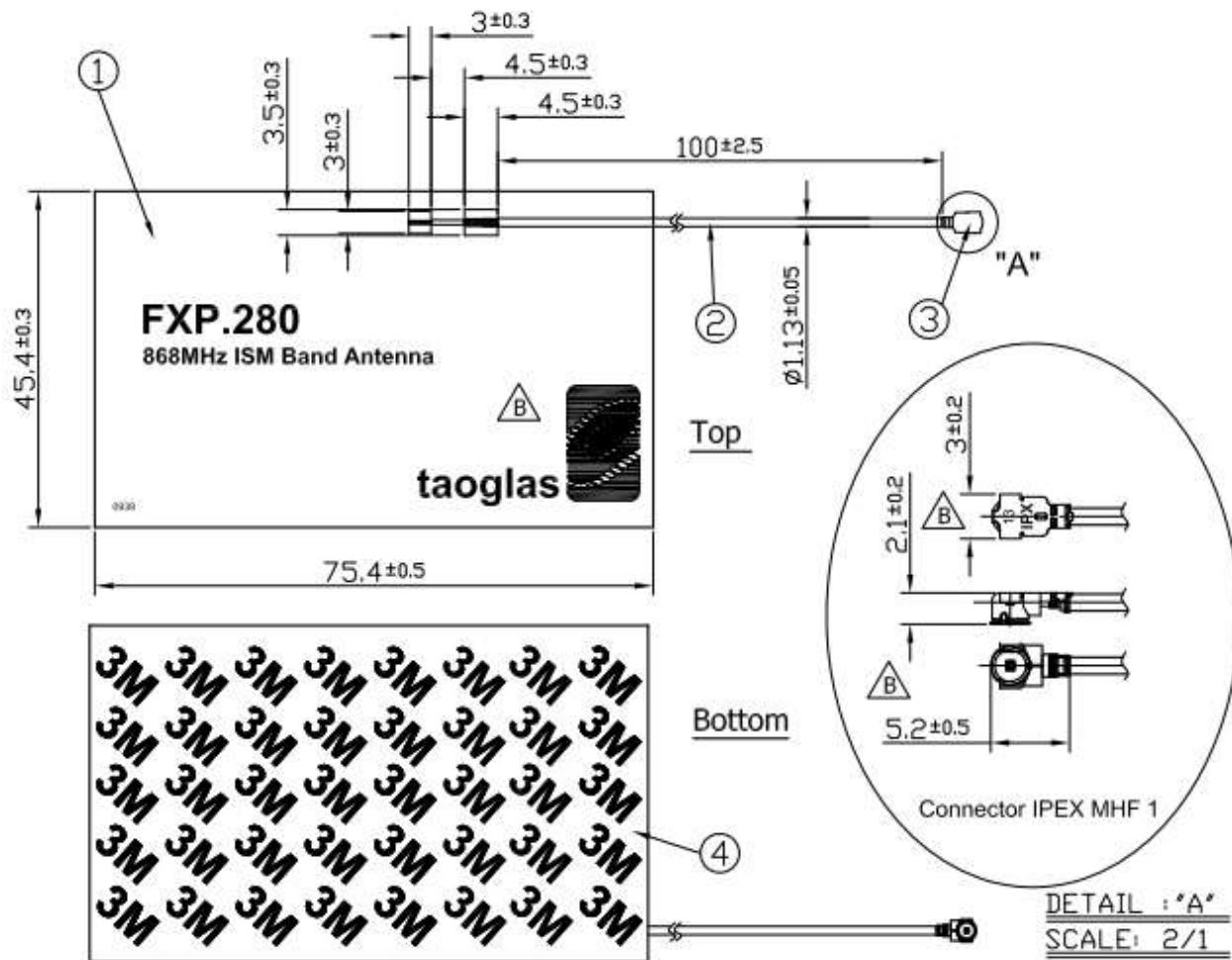
**Figure 12.** Mechanical Drawing for the FXP280 Antenna.
