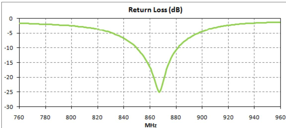
**Figure 3.** Return Loss for the FXP280 Antenna.
