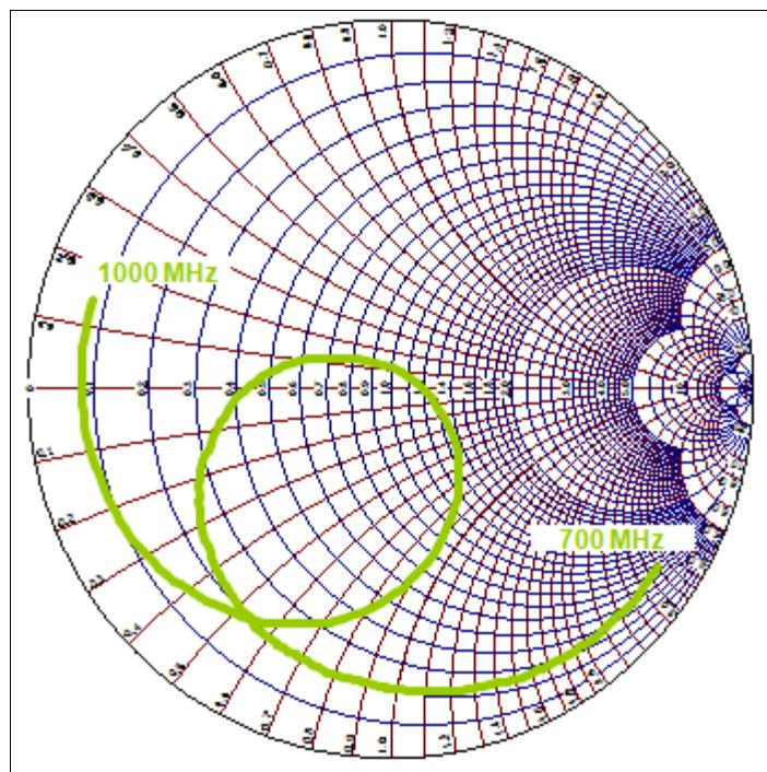
**Figure 5.** Smith Chart for the FXP280 Antenna.
