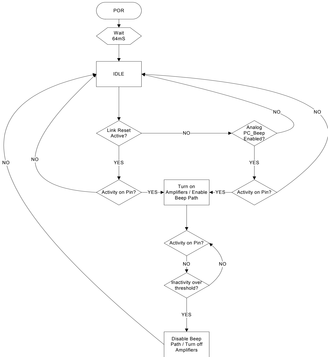
Figure 7. Analog PCBeep Flow Chart
