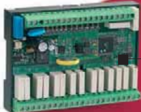
Millenium 3 expanded bare board with 16 relay outputs
