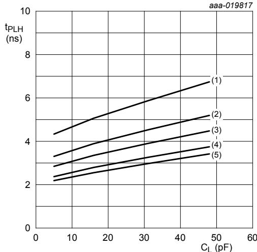
a. LOW to HIGH propagation delay (A to Y<sub>n</sub>);
