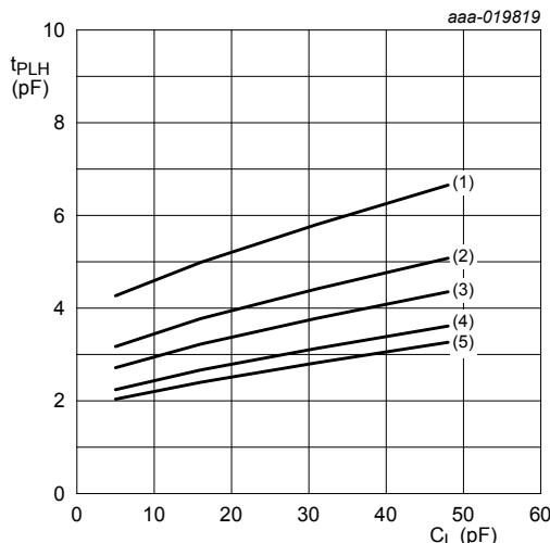
c. LOW to HIGH propagation delay (A to Y<sub>n</sub>);
