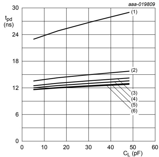
b. Propagation delay (A to  $Y_n$ );  $V_{CC(A)} = 0.8$  V
