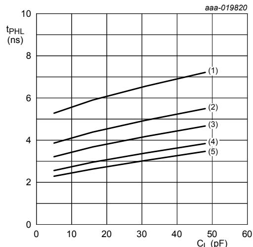
d. HIGH to LOW propagation delay (A to Y<sub>n</sub>);
