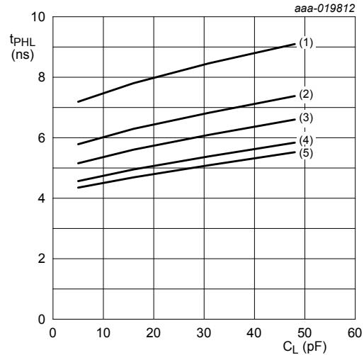
a. LOW to HIGH propagation delay (A to  $Y_n$ );  $V_{CC(A)} = 1.2$  V   b. HIGH to LOW propagation delay (A to  $Y_n$ );  $V_{CC(A)} = 1.2$  V
