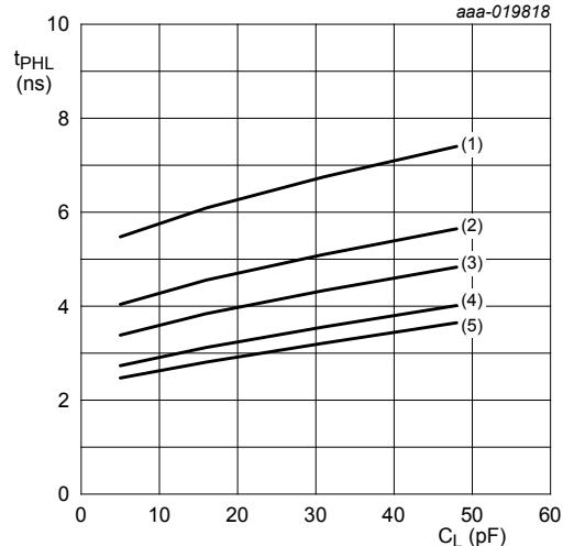
b. HIGH to LOW propagation delay (A to Y<sub>n</sub>);
