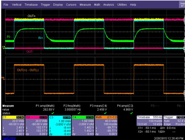
Figure 11. Floating Reference at 3 Hz and No Load
