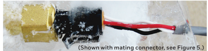
Figure 2. PX3 Series External Freeze/Thaw Resistance
