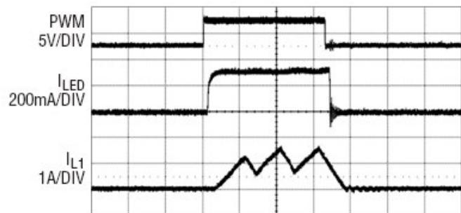
Figure 2. DC1279A 30V LED string PWM Dim, PVIN=12V
