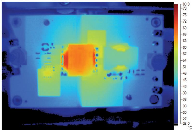
Figure 6. Thermal Map, Frontside at 48V<sub>IN</sub> and 12A<sub>OUT</sub> (T<sub>A</sub> = 25°C, 200LFM)
