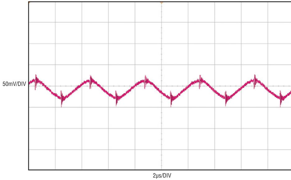
Figure 4. Output Ripple at 48V<sub>IN</sub> and 12A<sub>OUT</sub> (20MHz BW)
