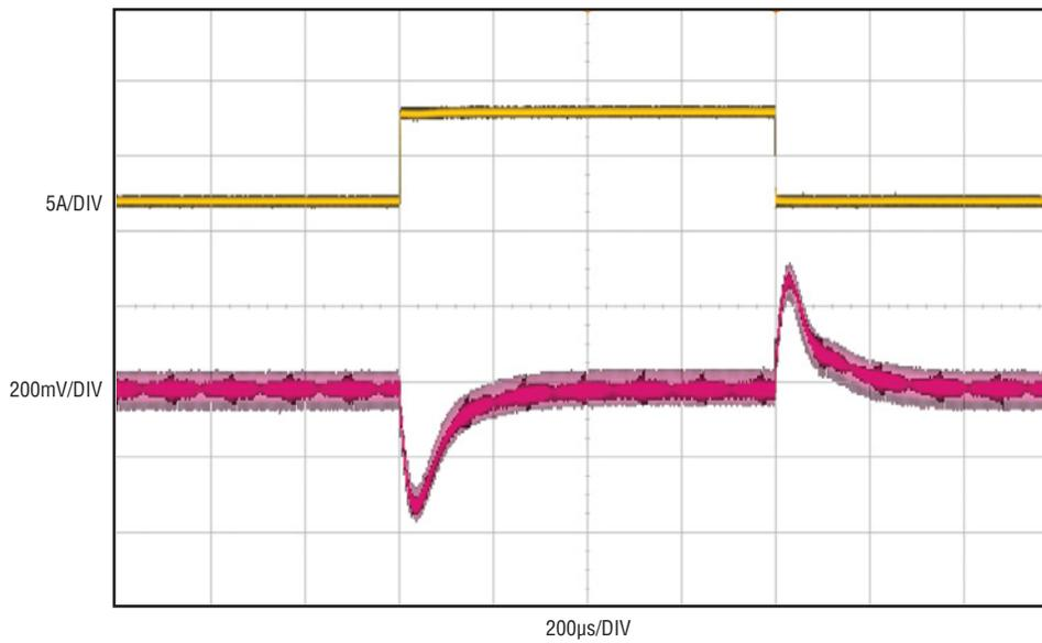
Figure 5. Load Transient Response Waveform at 48V<sub>IN</sub> and 6A<sub>OUT</sub> to 12A<sub>OUT</sub>
