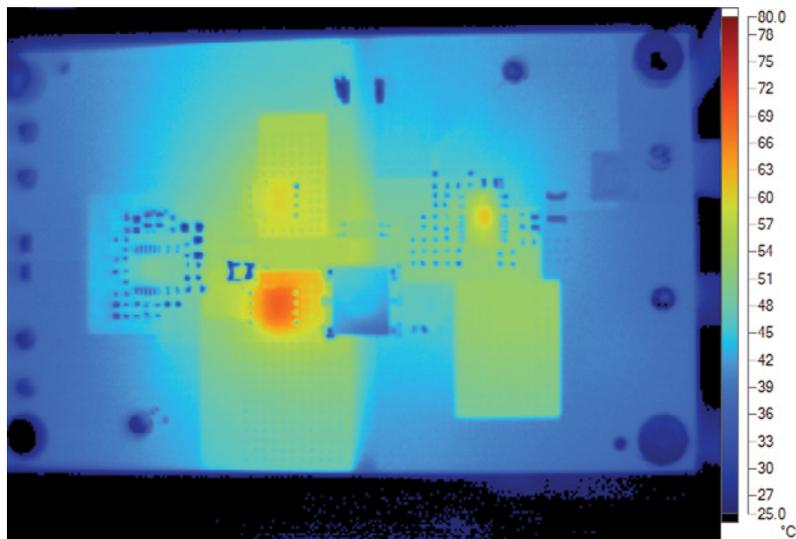
Figure 7. Thermal Map, Backside at 48V<sub>IN</sub> and 12A<sub>OUT</sub> (T<sub>A</sub> = 25°C, 200LFM)
