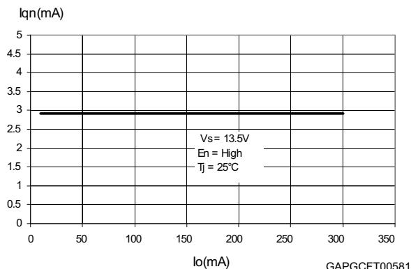
**Figure 8. Current consumption vs. output current (at light load condition)**
