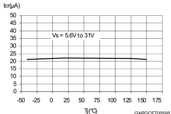
**Figure 22.  $I_{dr}$  vs  $T_j$**
