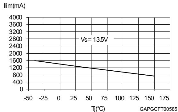
**Figure 12. Current limitation vs input voltage**
