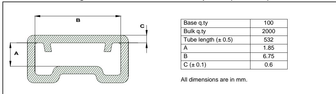
**Figure 34. PowerSSO-12 tape and reel shipment (suffix "TR")**
