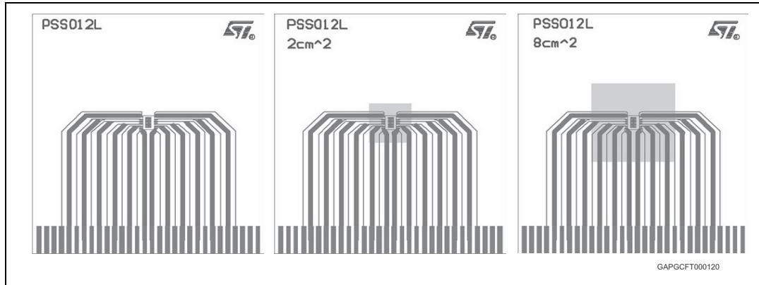
1. Layout condition of  $R_{th}$  and  $Z_{th}$  measurements (PCB: double layer, thermal vias, FR4 area = 77 mm x 86 mm, PCB thickness = 1.6 mm, Cu thickness = 70  $\mu$ m (front and back side), thermal vias separation 1.2 mm, thermal via diameter 0.3 mm +/- 0.08 mm, Cu thickness on vias 0.025 mm, Footprint dimension 4.1 mm x 6.5 mm ).
