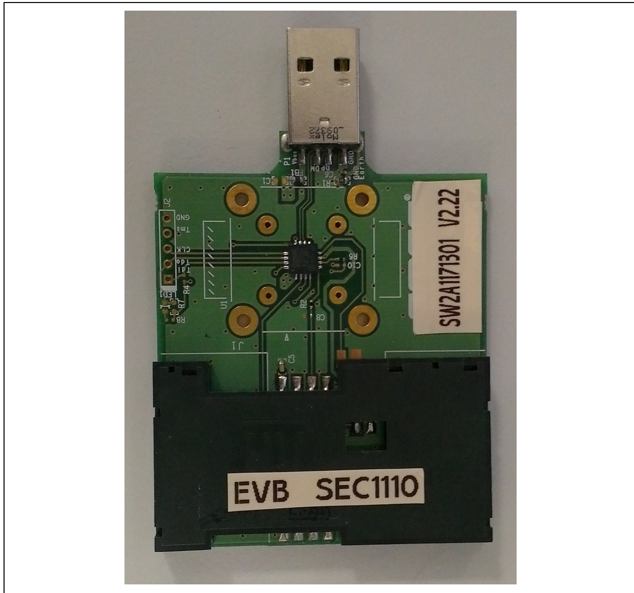
FIGURE 2-6: EVB-SEC1110 COMPONENT SIDE TOP LAYER
