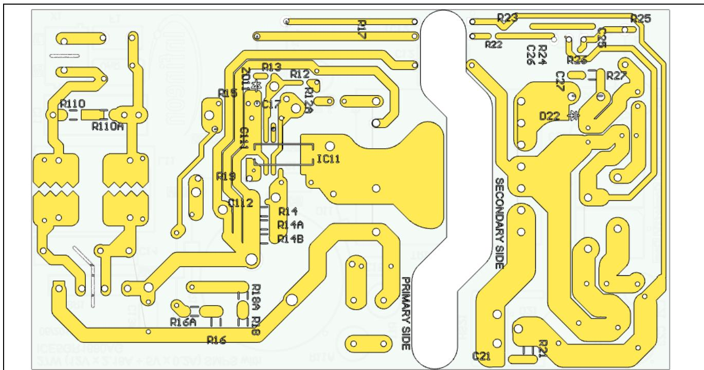
Figure 6 Bottom side copper and component legend
