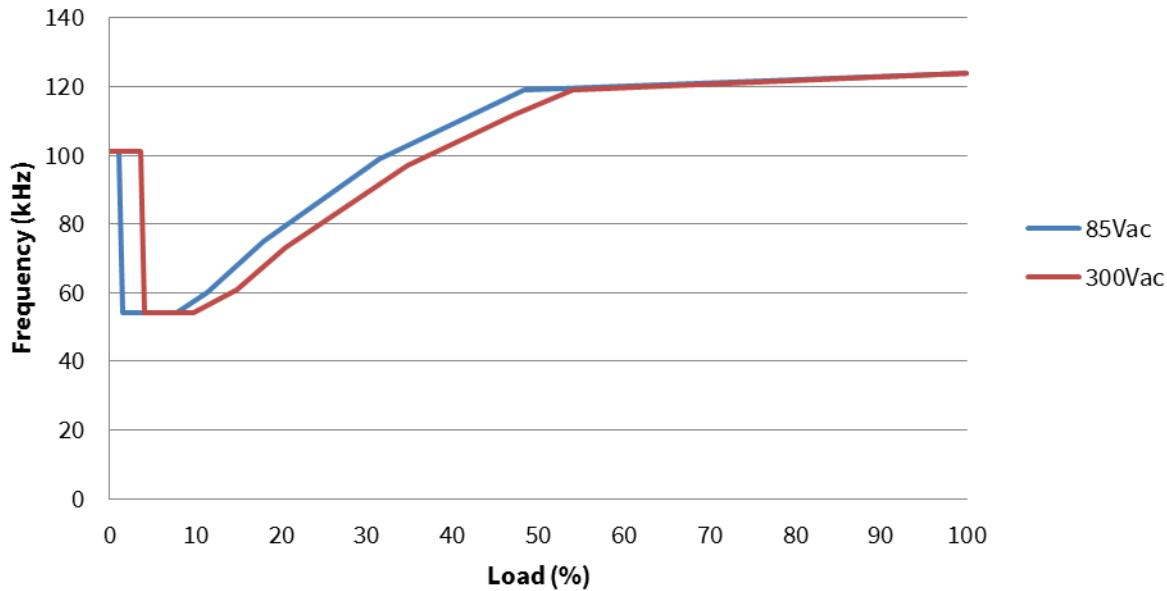
Figure 3 Frequency-reduction curve of DEMO\_5GR1680AG\_27W1
