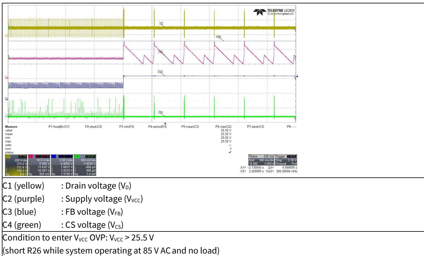
Figure 29 V<sub>VCC</sub> OVP
