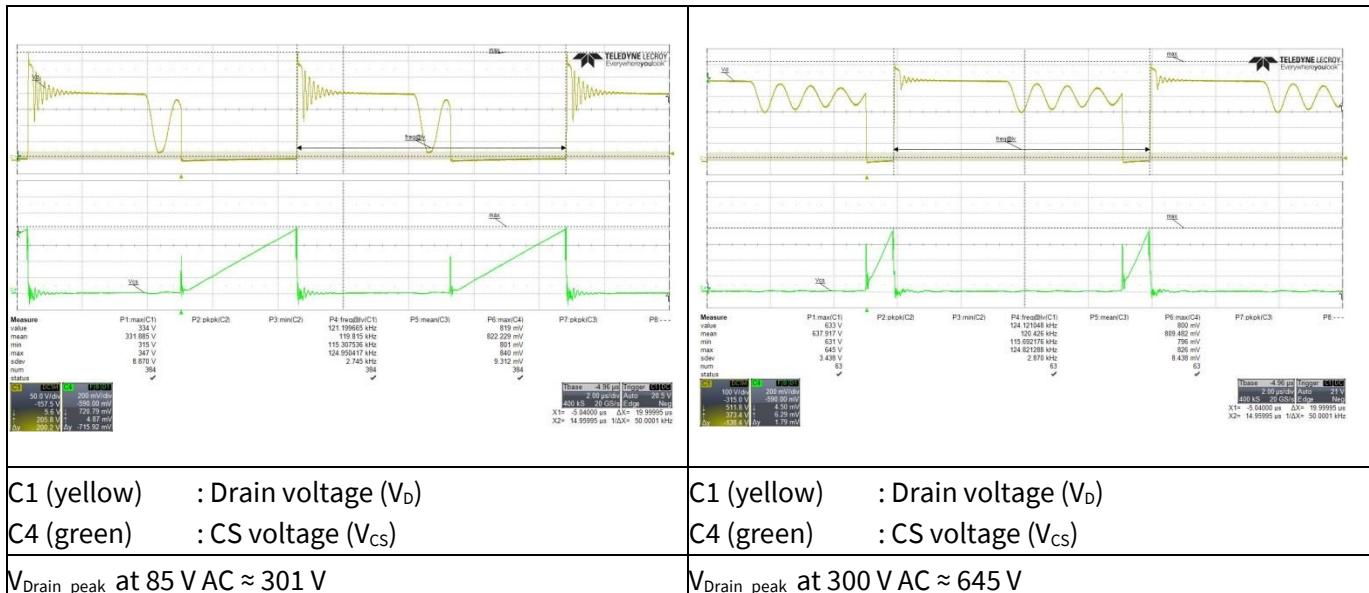
Figure 20 Drain and CS voltage at maximum load
