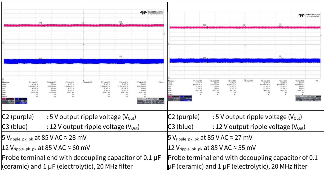
Figure 23 Output ripple voltage at maximum load
