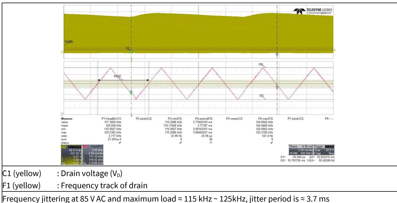
Figure 21 Frequency jittering
