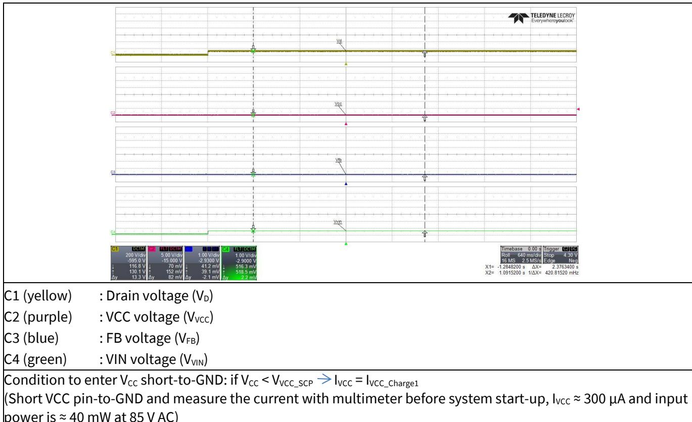
Figure 32 V<sub>CC</sub> short-to-GND protection
