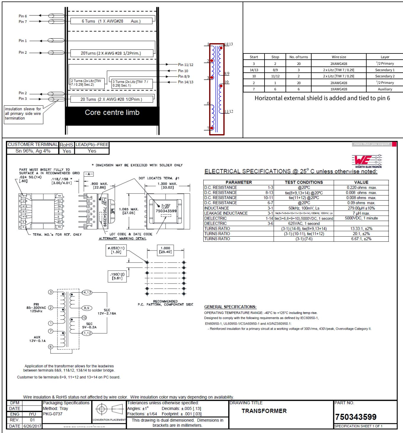
Figure 7 Transformer structure
