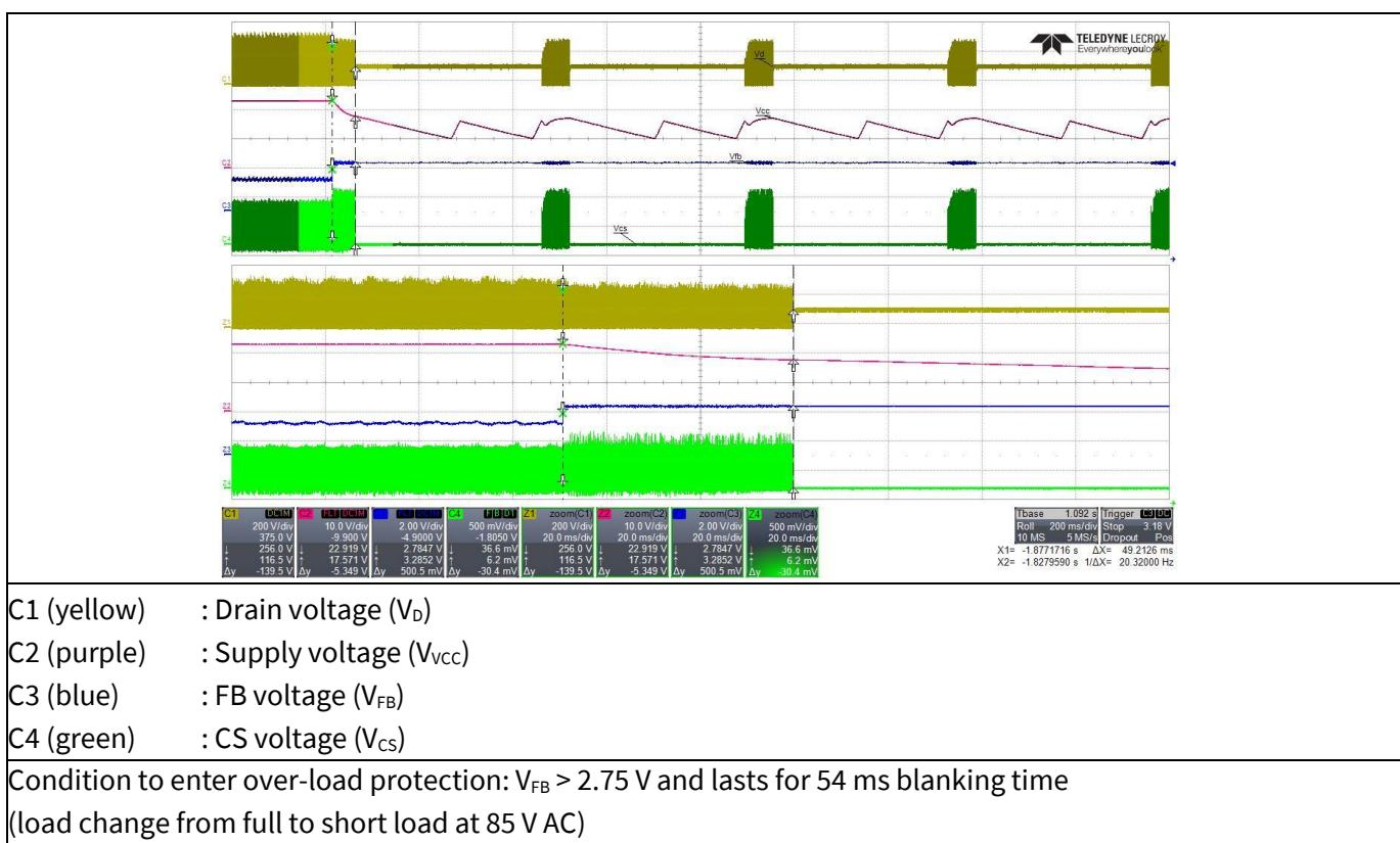
Figure 31 Over-load protection
