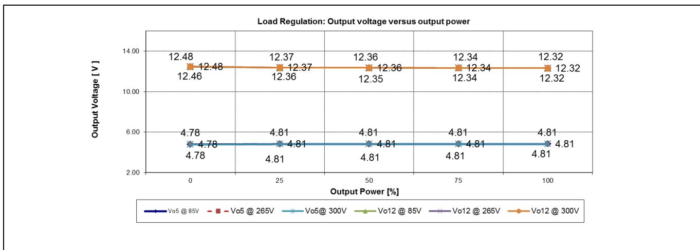
Figure 11 Load regulation  $V_{out}$  vs output power
