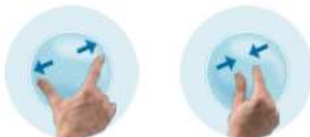
Figure 59 – Pinch/Stretch Multitouch Gestures
