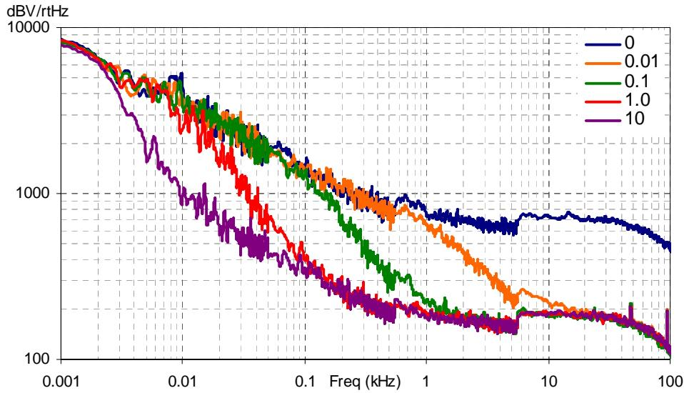
**Figure 3-9. Typical AGND Noise with P2[4] Bypass**
