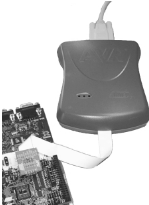
Figure 1-4. Emulating with JTAG ICE
