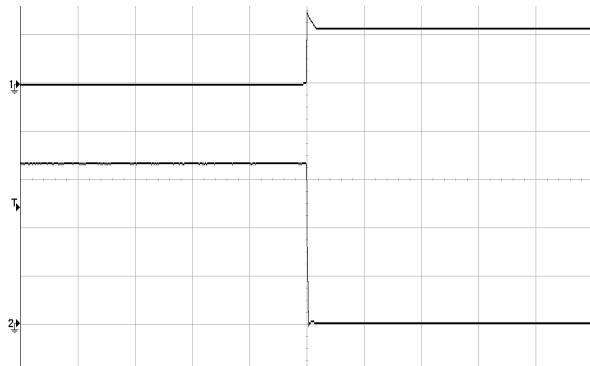
Figure 10 Output voltage shutdown by remote OFF, (5ms/div), see Figure 11 for test configuration; CH1-remote OFF voltage (5V/div); CH2-output voltage (1V/div)
