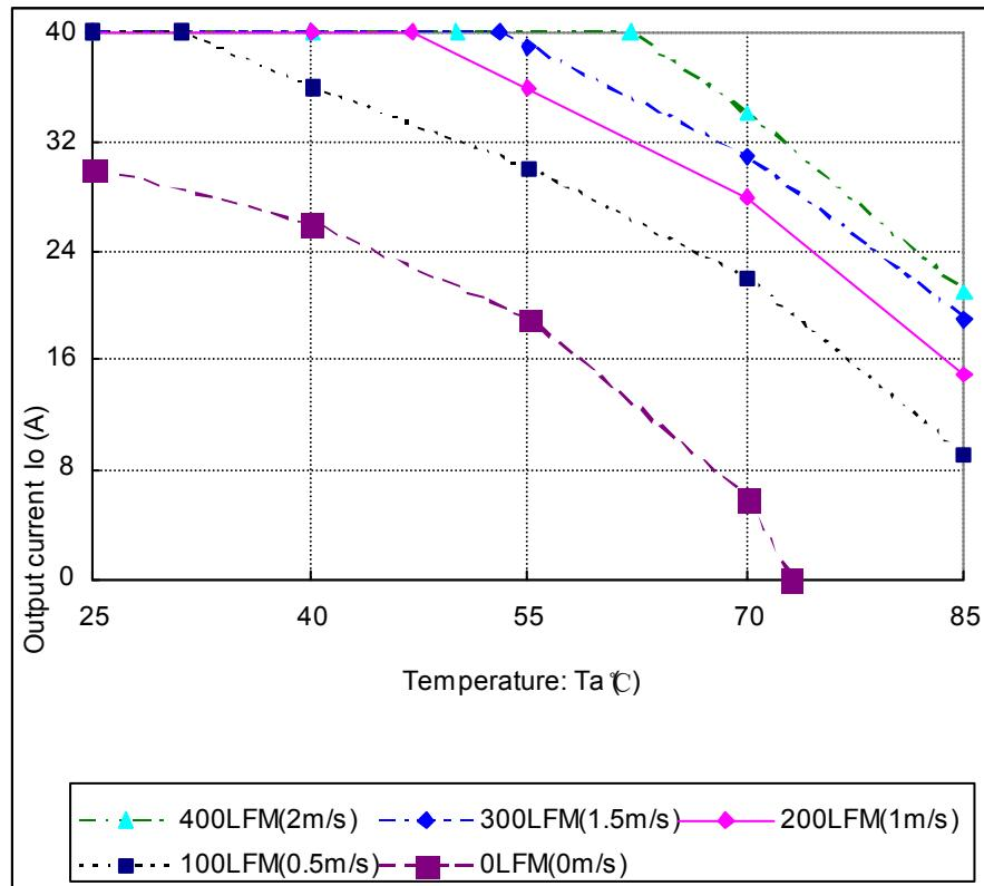
Figure 2 Output power derating,  $48\text{V}_{\text{in}}$ , air flowing across the converter from pin 1 to pin 3
