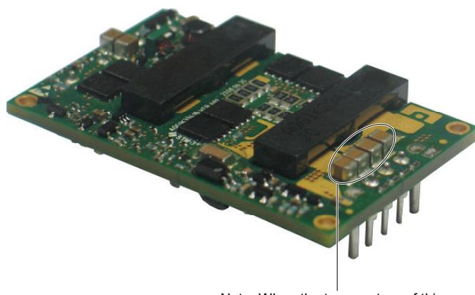
Note: When the temperature of this test point is lower than 100°C, the module thermal reliability is available
