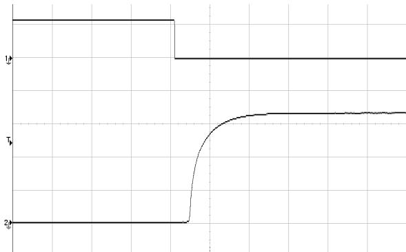
Figure 9 Output voltage startup by remote ON, (5ms/div), see Figure 11 for test configuration; CH1-remote ON (5V/div); CH2-output voltage (1V/div)
