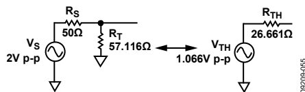
Figure 48. Thevenin Equivalent Circuit
