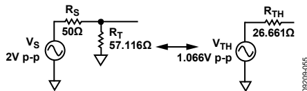
Figure 48. Thevenin Equivalent Circuit
