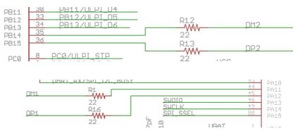
If higher file access speed is desired, a ULPI PHY (for example FUSB2805) can be added on USB1 port, which will change the USB interface to High-Speed bus (480Mbps).
