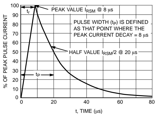
Figure 11. 8 × 20 μs Pulse Waveform
