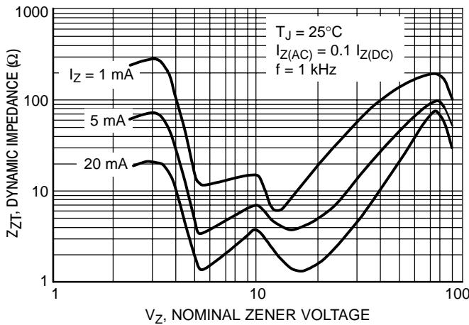
**Figure 5. Effect of Zener Voltage on
