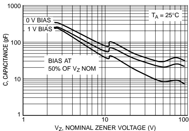
Figure 7. Typical Capacitance
