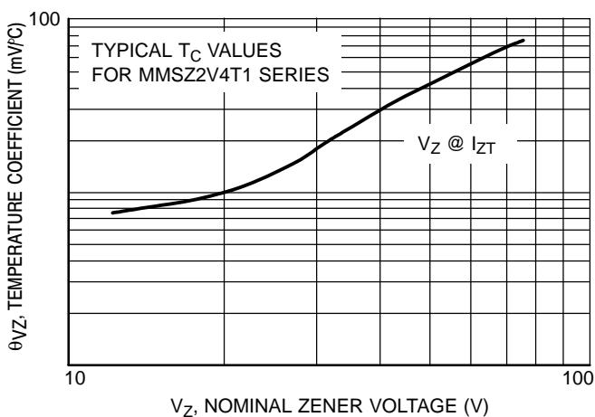
**Figure 2. Temperature Coefficients
