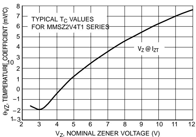
**Figure 1. Temperature Coefficients
