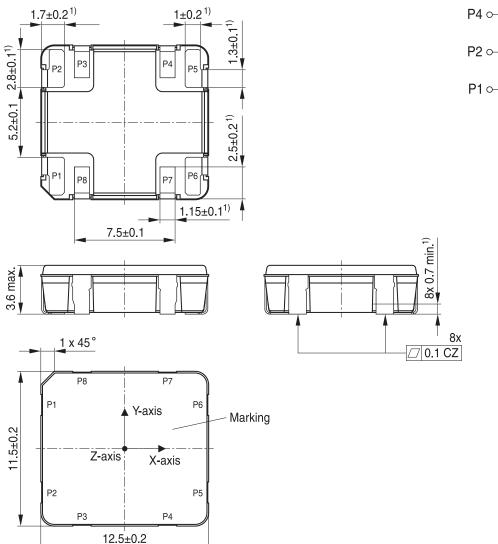
1) Soldering area Dimensions in mm
