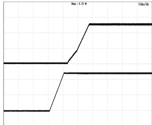
Figure 4: Input Voltage Start-up at full load V_{in}=48V , I_{out}=6A Time: 50ms/div. V_{out} (top trace): 20V/div; V_{in} (bottom trace): 20V/div.
