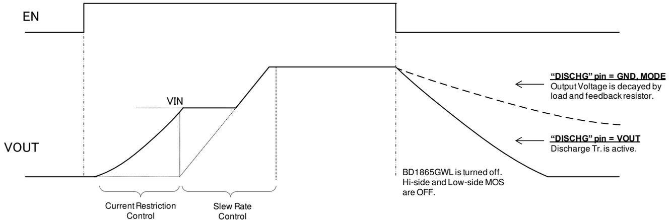
Figure. 23 Start-up (Soft Start) and Shutdown Operation
