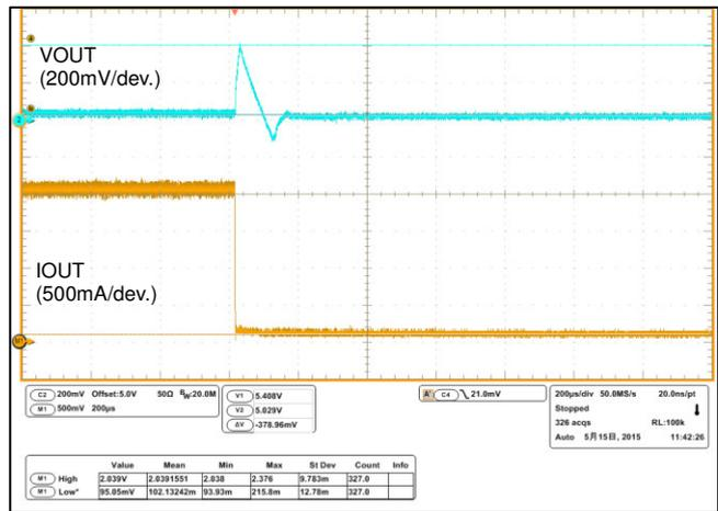
Figure. 13 Transient Response (PFM/PWM mode)
