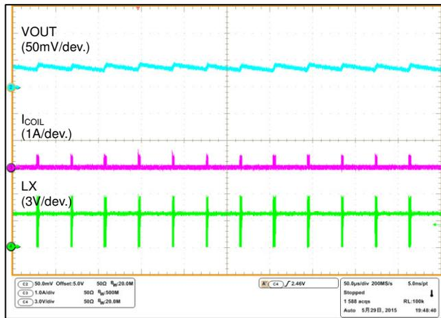
Figure. 18 Operation Waveform (Mixing-PWM)
