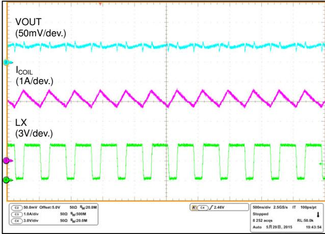
Figure. 16 Operation Waveform (PWM)
