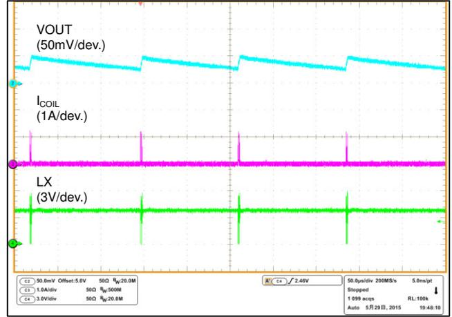
Figure. 17 Operation Waveform (PFM)
