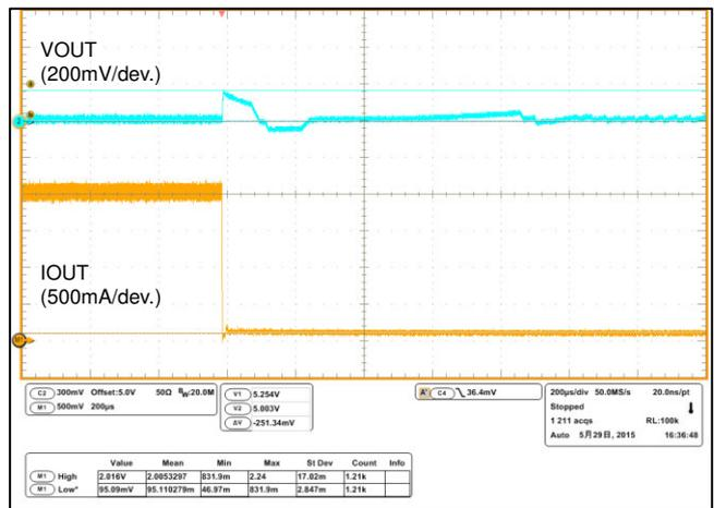
Figure. 15 Transient Response (Mixing-PWM mode)
