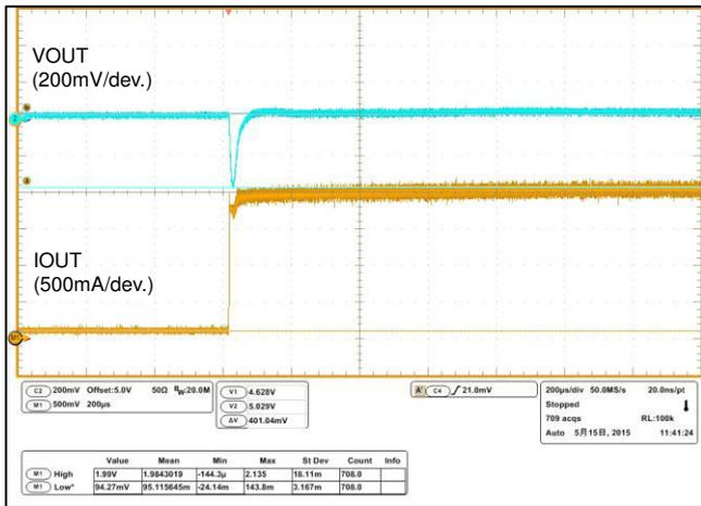
Figure. 12 Transient Response (PFM/PWM mode)
