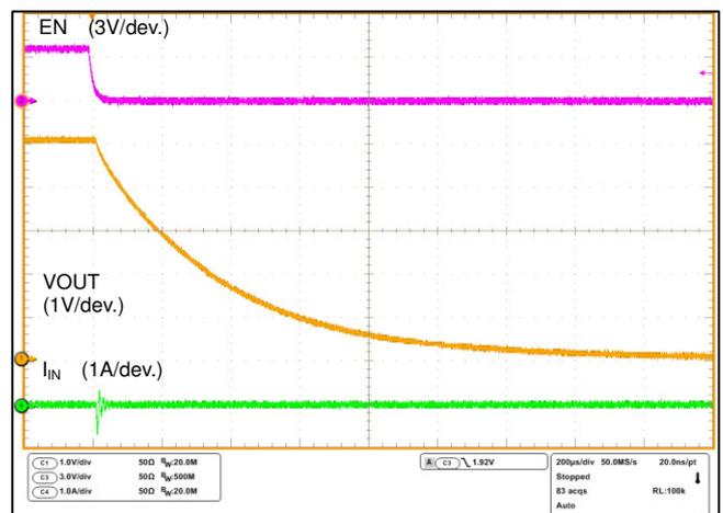
Figure. 21 Shutdown Waveform  $I_o = 0A$
