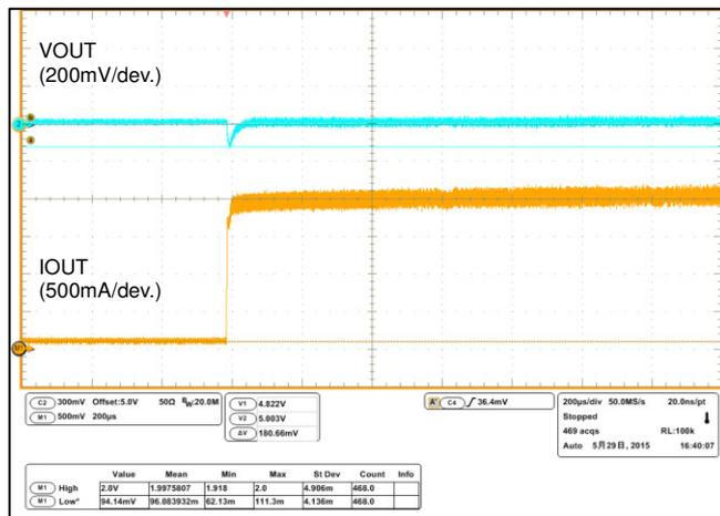
Figure. 14 Transient Response (Mixing-PWM mode)
