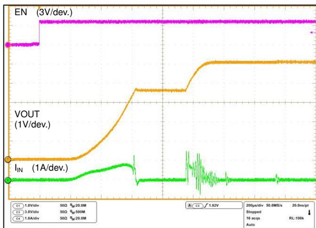
Figure. 20 Start-up Waveform (Soft-Start)  $I_o = 0A$
